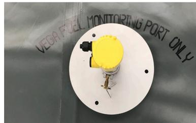
*VEGA Fuel Monitoring System Stabilising Plate*
