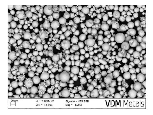
The picture shows a typical micrograph of VDM $^{\! \odot}$  Powder 718 CTP as an example.
